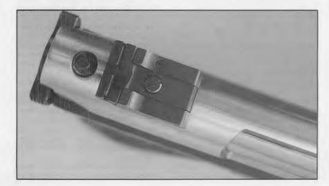
Point the muzzle up and pull the trigger to make sure the hammer is still cocked. Slide the bolt group into the receiver.
